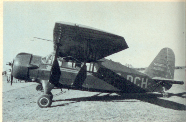
The last Skyrocket model—a 31-55A built by Northwest Industries, Edmonton, Alberta, Canada, after World War II. This model was designed for full NACA cowling around the Wasp engine. The single-strut landing gear dates from 1934.
